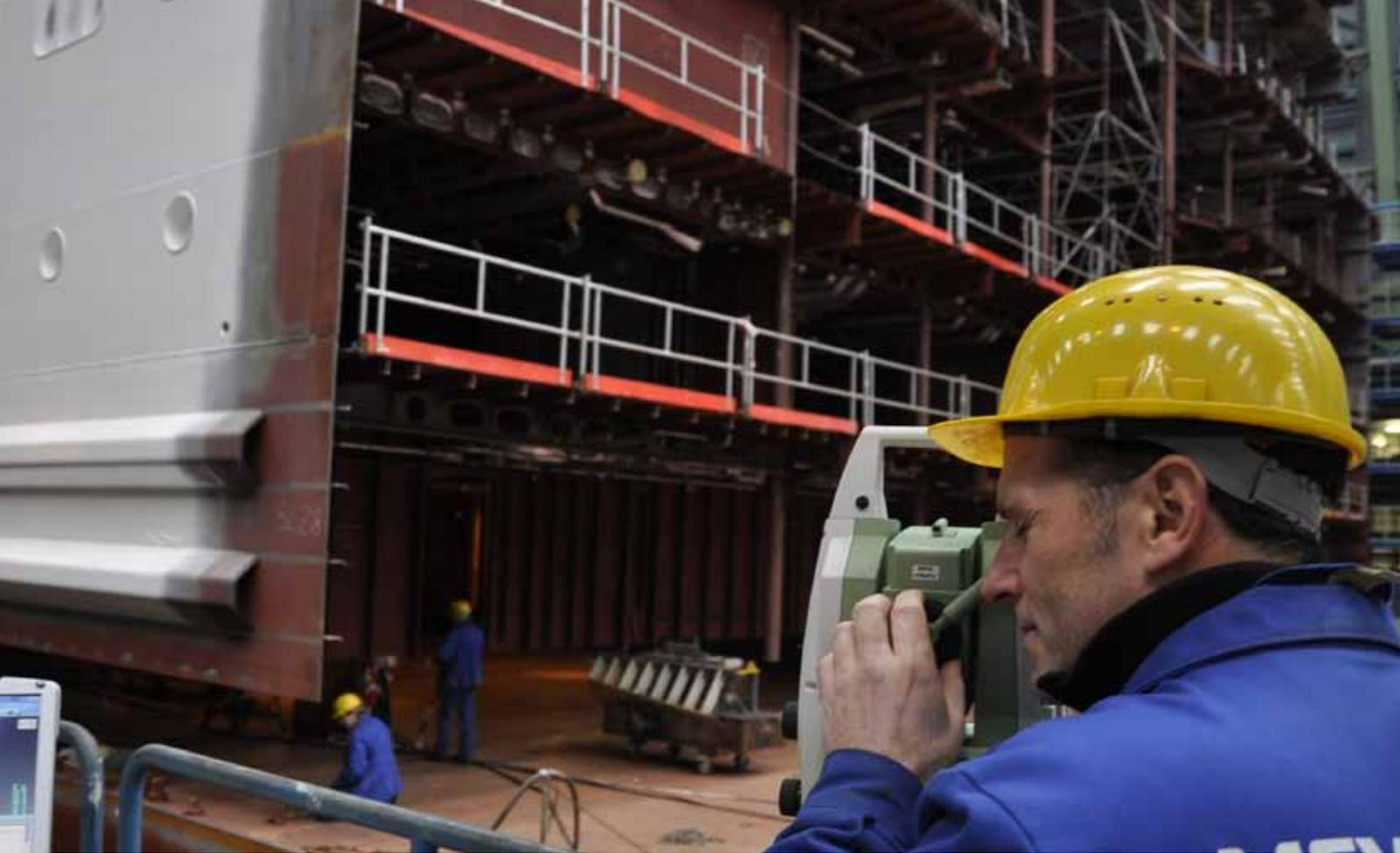
*Precisely positioning 800 tonnes of steel: laying the keel of a block for the Celebrity Silhouette.*
