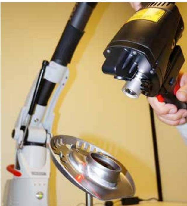
The ROMER Absolute Arm SI is a highly profitable laser scanner solution. The ability to scan without having to calibrate the equipment or set the laser according to part reflectivity or colour gives enormous versatility.
