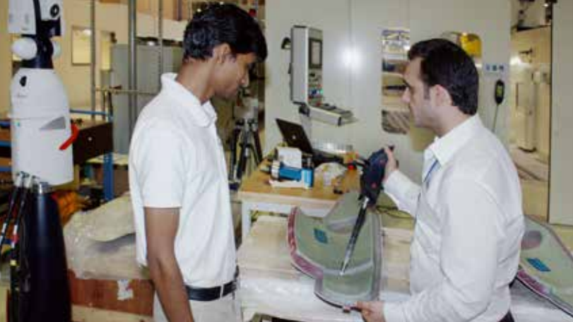
Part/surface inspection with Leica Absolute Tracker AT901 with Leica T-Probe
