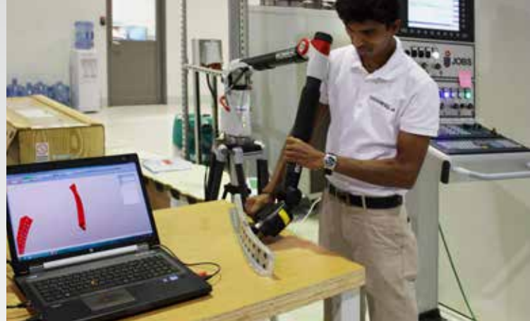
Inspection of fixtures with ROMER Absolute Arm
