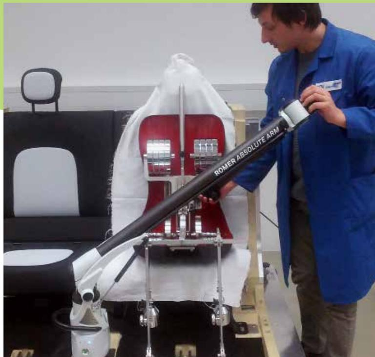
The position of vehicle occupants in their seats is assessed against strict safety standards by using the ROMER Absolute Arm to measure dummies seated in the car.
