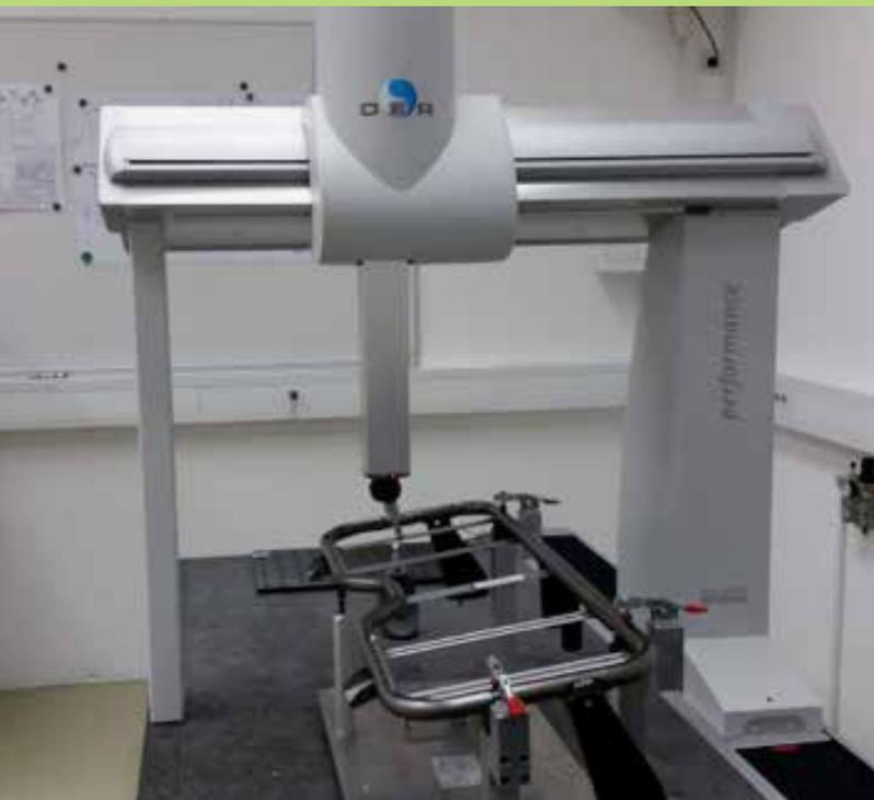
Measurement of the steel seat frame using the DEA GLOBAL Silver Performance CMM from Hexagon Metrology.
