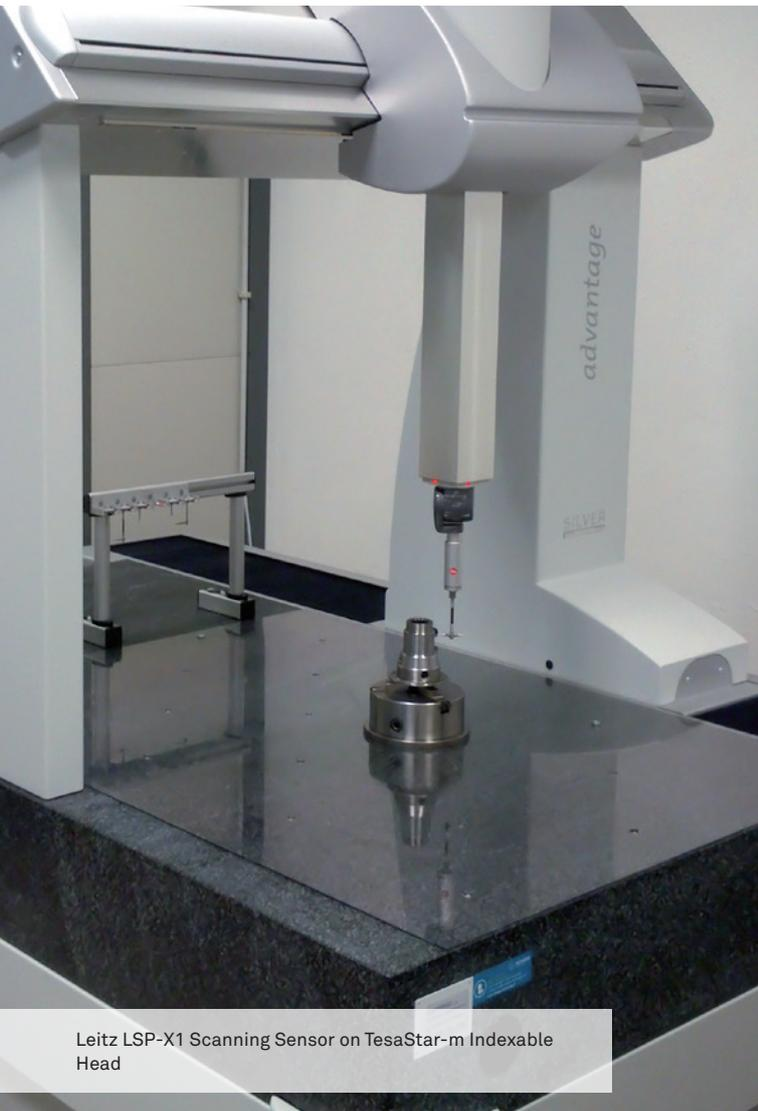
Leitz LSP-X1 Scanning Sensor on TesaStar-m Indexable Head
