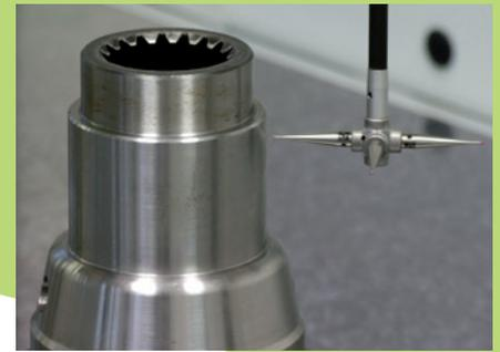
“A measuring machine is a general purpose tool that allows you to inspect not only the gear tooth characteristics, but also the geometry of drive shafts and wheels – all with a single system.”
