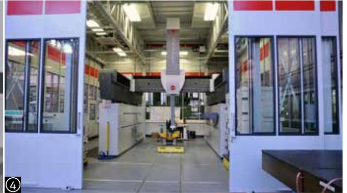
① Hexagon Metrology designed the entire Leitz PMM-G package: measuring machine and software, air-conditioned measuring room and feeding system. ② Optimum measurement precision is achieved even with long and heavy sensors. ③ Measuring a ram with the Leitz PMM-G. ④ The reinforced concrete base body ensures minimal mass movements.
