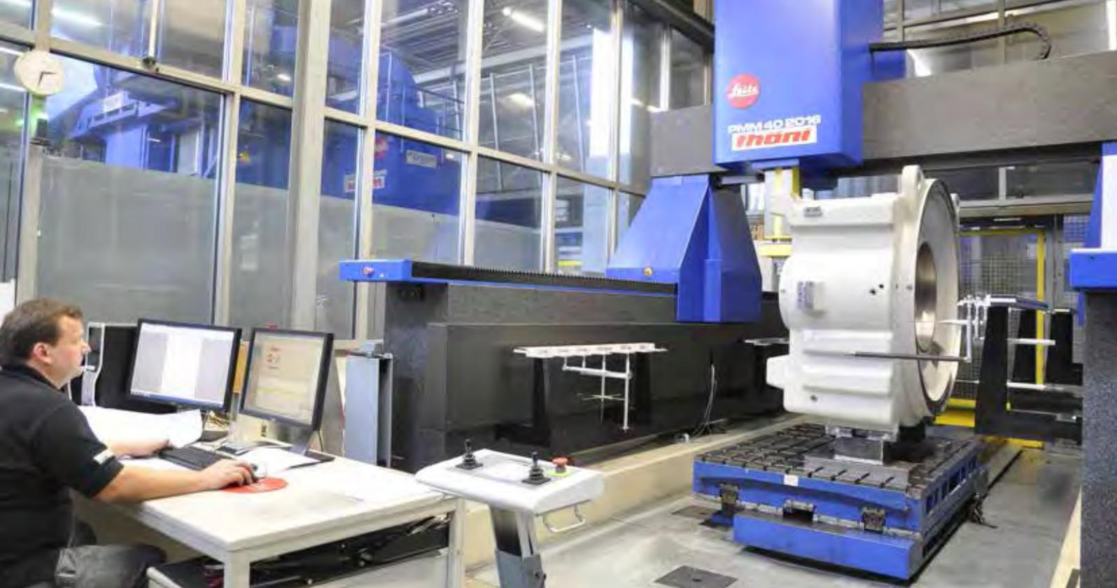
*The overhauled Leitz PMM precisely measures the regular shapes of wind turbine housings weighing many tonnes.*
