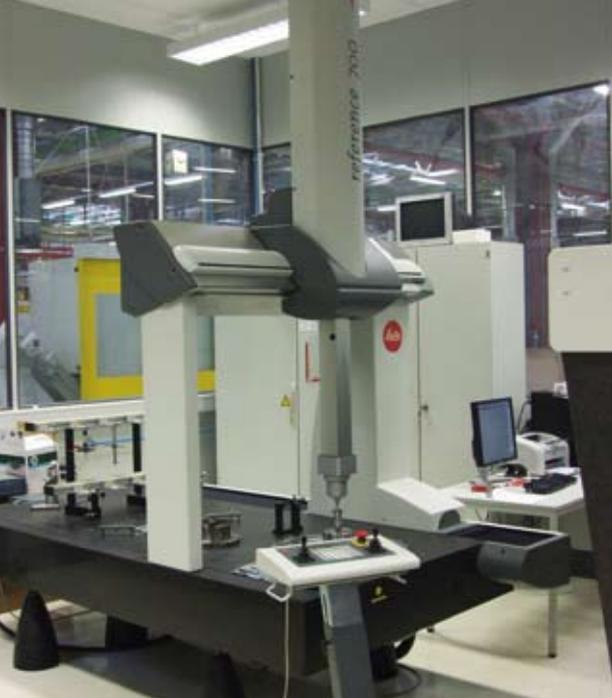
*A total of three Leitz Reference belong to the measuring inventory. On two of these coordinate measuring machines the cam units and basic shafts are tested.*
