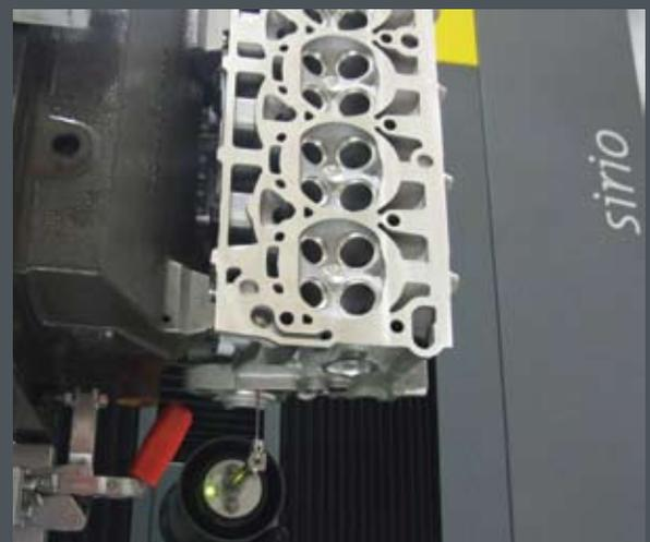
*Complex parts like this cylinder head of the Global Engine are measured from a Leitz SIRIO. The SIRIO MultiScan offers speed and flexibility.*
