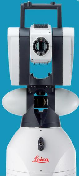
**The project at hand integrated a laser tracker with a robot in order to develop and solve the kinematic calibration of the robot, and integrate the laser tracker measurements as feedback controlling the position and orientation of the drill head. The purpose of the project was to evaluate whether flexible robot systems can deliver precise DA hole patterns within aerospace tolerances.**
