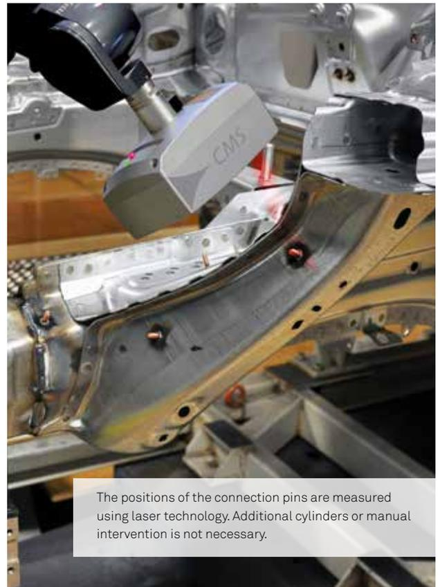
The positions of the connection pins are measured using laser technology. Additional cylinders or manual intervention is not necessary.
