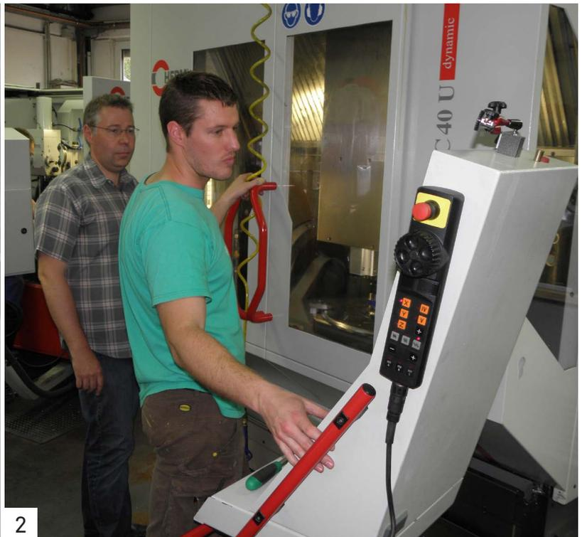
1| 3D Form Inspect makes it possible to check the nominal and actual geometry in the machine and, if necessary, immediately re-work in the same clamping arrangement. 2| With 3D Form Inspect the operator and supervisor always have an overview of the accuracy.
