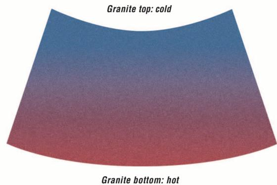
***Granite’s low coefficient of thermal conductivity results in slow heat conduction which can result in large thermal gradients within a thick slab of granite. As shown in the illustration (exaggerated for clarity), this causes the granite to bend as the opposing surfaces expand or contract differently. Aluminum on the other hand quickly conducts heat due to its much higher coefficient of thermal conductivity, thus avoiding thermally induced geometric distortion.***
